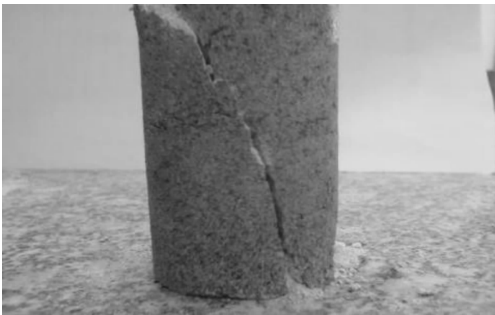
图 4 三轴试验破坏形态 Fig. 4 Triaxial compressive test failure forms
