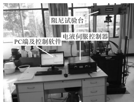
图4 减振器试验台系统 Fig. 4 Test bench system of shock absorber
