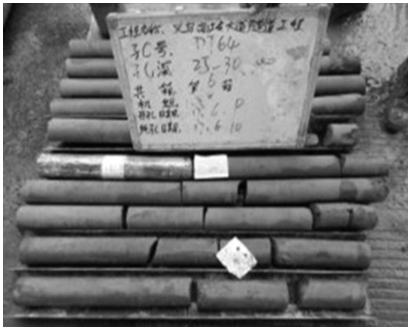
图 1 中风化泥质粉砂岩取样照片 Fig. 1 Sampling photo of middle-weathered argillaceous siltstone
